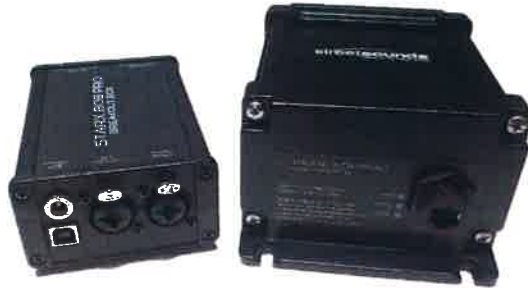
BOB Pro Indoor Unit and STARX Transceiver Outdoor Unit
