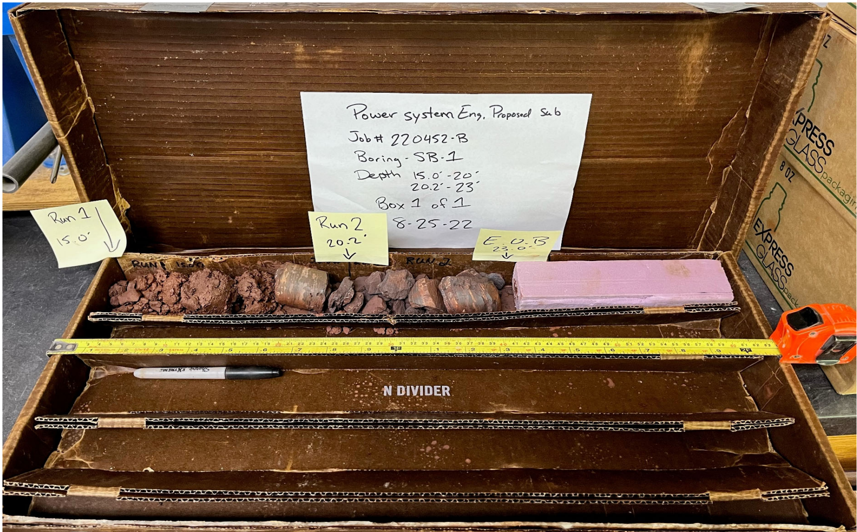
Boring SB-1 Depth 15.0' - 20.0' and 20.2' - 23.0'
